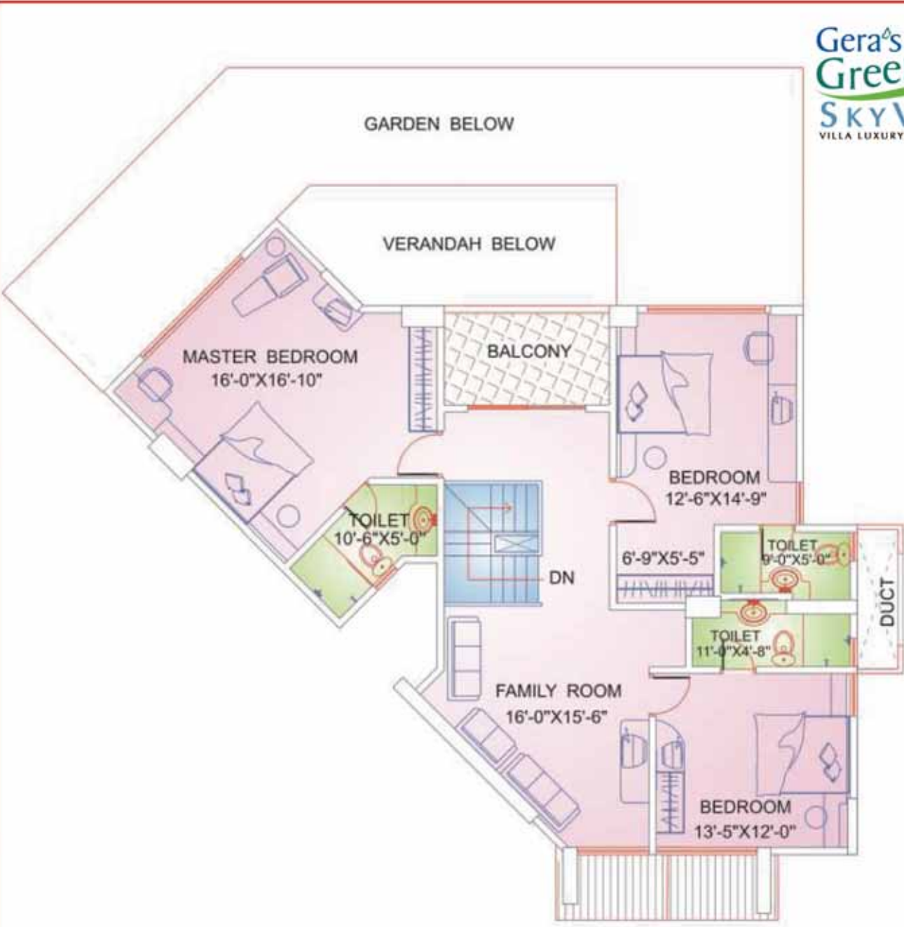
Upper Level - End Unit Ground Floor Plan Building No. III, IV & V
